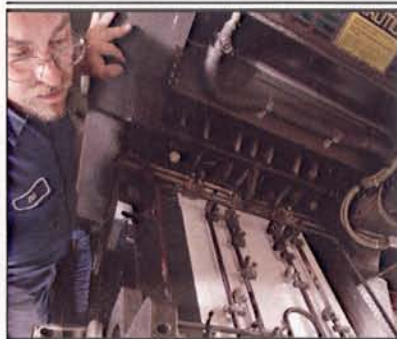
A two-unit Heidelberg found new life with interstation curing and printing with UV inks on plastics for a variety of products produced by Datalizer at its plant in Addison, IL, near Chicago.
