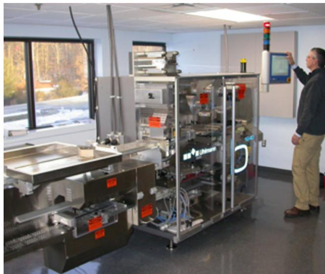
*Figure 3: Uhlmann B 1240 blister machine produces testable quality blisters rapidly.*
