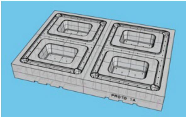
Figure 1: 3-D CAD model of a forming tool for a blister pack
