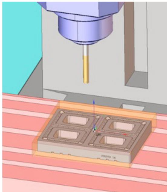
Figure 2: Digital dry run of form tool machining process
