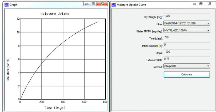
Figure 7: MVTR uptake plot for a sample pharmaceutical, with inputs on the right.
