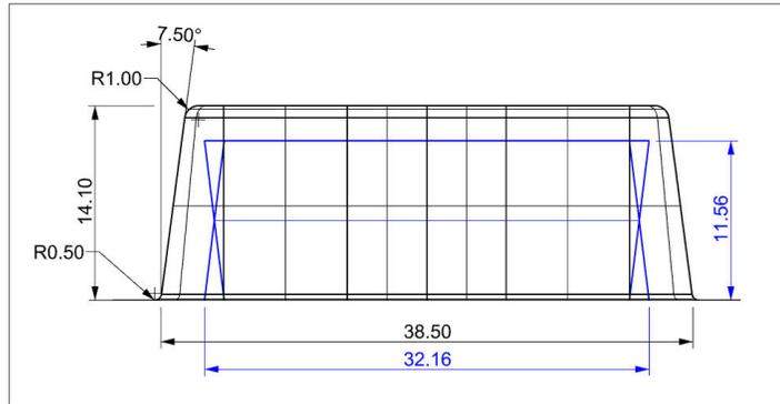
Figure 1: Preliminary CAD design for a blister cavity holding a trapezoidal lozenge.
