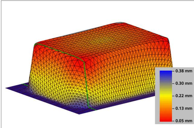
Figure 3: Contour map of provisional cavity design for a sample product.
