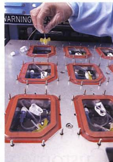
The tubing coils neatly, with no kinks, in a recess. More important, the needle can be removed the same way, each and every time.
