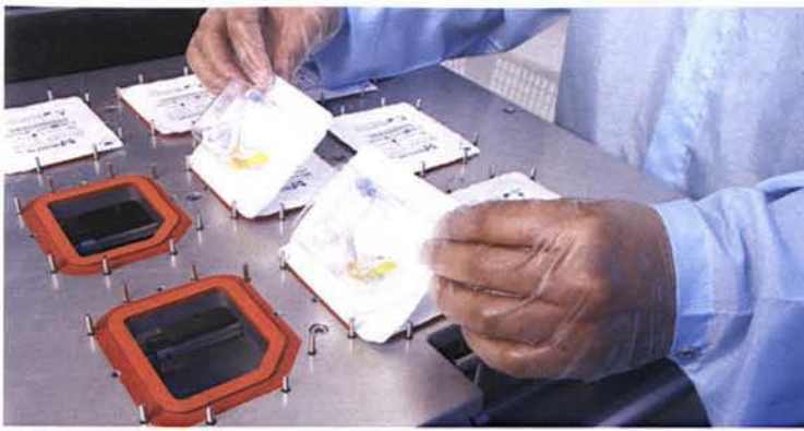
The narrow thermoforming cavity maintains material distribution to the bottom with a 'rib' along one wall that supports the product.
