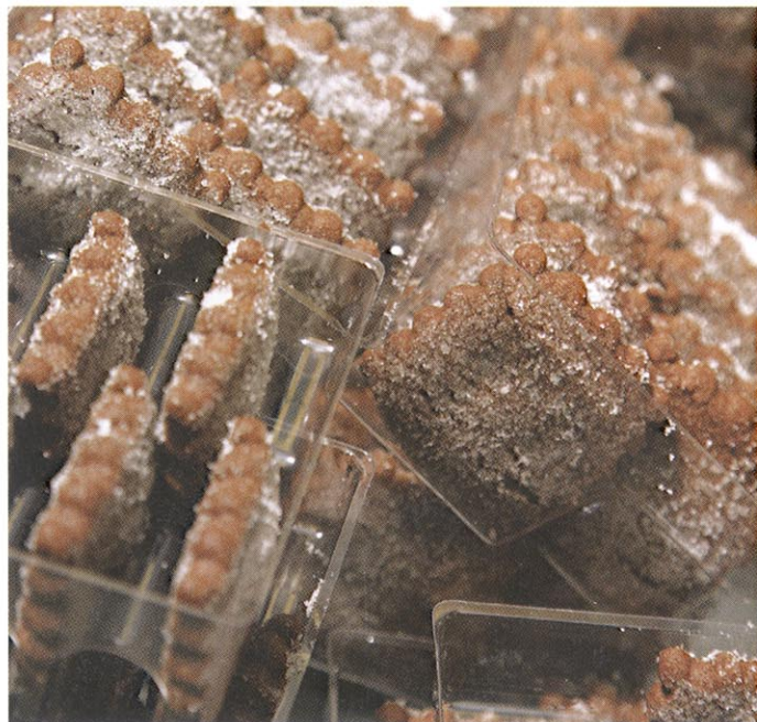
STAGGERING DESIGN. The new tray design staggers the cookies slightly to keep them from touching and rubbing off their coatings.
