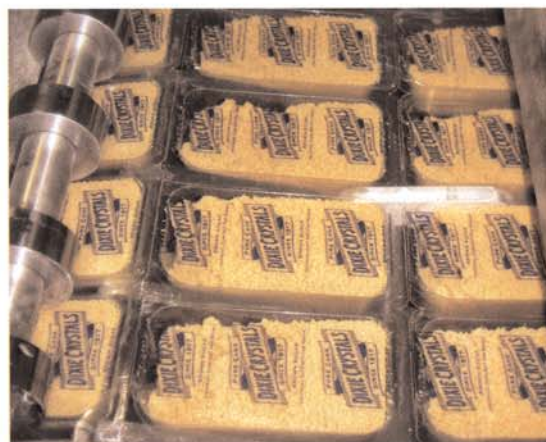
Rotary knives cut freshly produced packs from their web.
