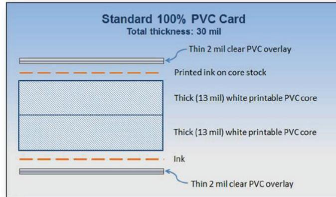
**Figure 2: Industry standard, 100% PVC card structure.**
