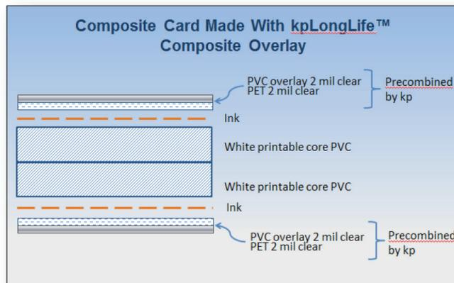
**Figure 4: Composite card made with Pentacard® kpLongLife™ 2+2 film with 4 mil composite overlay (2 mil per side).**
