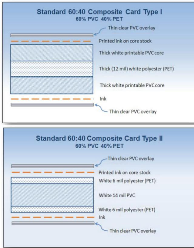
**Figure 3: Two versions of the industry standard 60:40 high durability card structure.**
