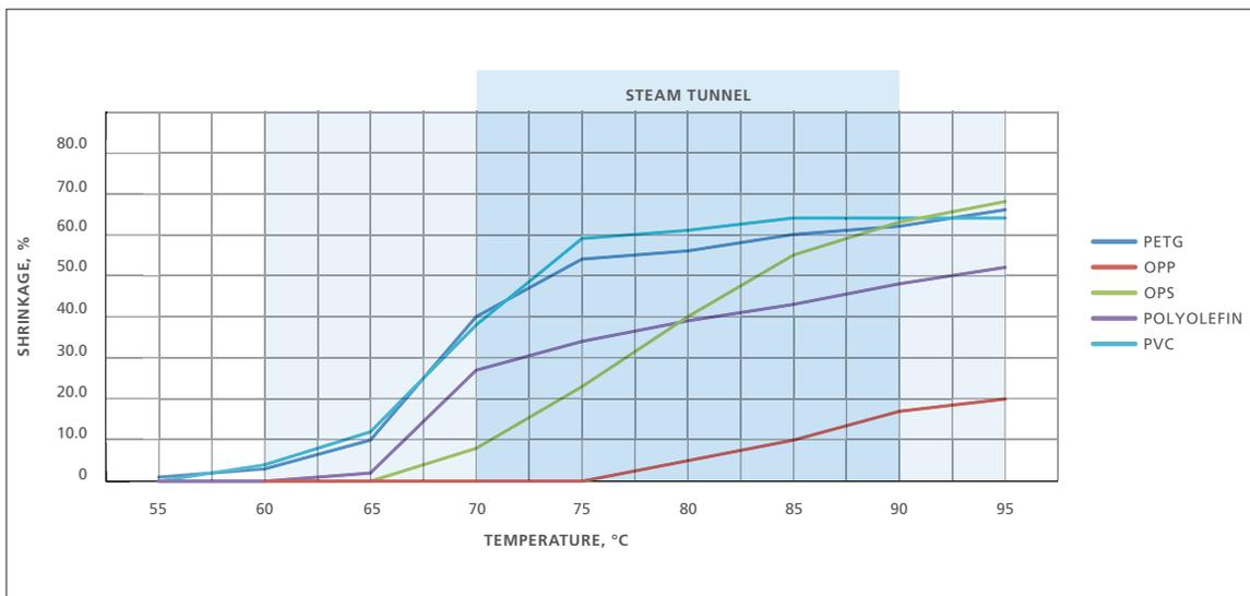
*Note: Blue shaded area indicates typical steam tunnel operating temperatures*
